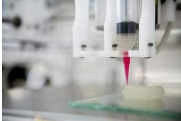
A 3-D printer in Weill Hall at Cornell University deposits cells encapsulated in a hydrogel that will develop into new ear tissue. The printer takes instructions from a file built from 3-D photographs of human ears taken with a scanner in Rhodes Hall. / Lindsay France / Cornell University photo
