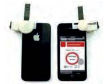
The Cornell NutriPhone prototype. A test strip containing a saliva or sweat sample is loaded into the slot, photographed, and then analyzed for health purposes. Image provided.
